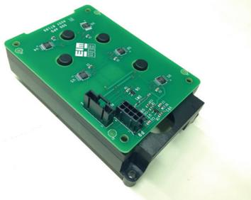
**Absolute Position Detector** provides precise valve position under all conditions including loss of power, no battery backup required.
