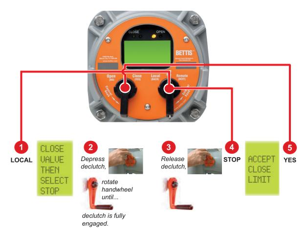
Turn the selector knob to the LOCAL position. At the "CLOSE VALVE THEN SELECT STOP" prompt, depress the declutch lever while rotating the handwheel until the clutch is fully engaged. Release the lever. When the valve is fully closed. Return the selector knob to the STOP position. At the "ACCEPT CLOSE LIMIT" prompt, select "YES."
