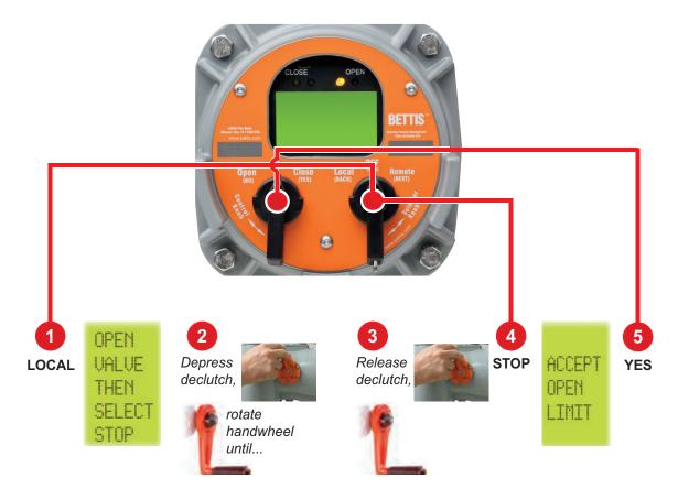
Turn the selector knob to the LOCAL position. At the "OPEN VALVE THEN SELECT STOP" prompt, depress the declutch lever while rotating the handwheel until the clutch is fully engaged. Release the lever. When the valve is fully opened. Return the selector knob to the STOP position. At the "SAVE LIMITS" prompt, select "YES."
