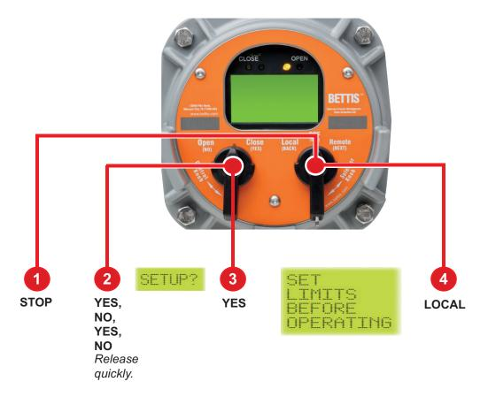
Place the selector knob in the **STOP** position. Then toggle the control knob in rapid succession to **YES**, then **NO**, then **YES**, then **NO** and release. The Setup icon will be displayed on the display module and **"SETUP?"** will be displayed on the message center. Rotate the control knob to **"YES."** The message center will display **"SET LIMITS BEFORE OPERATING."** Set position limits as described on the next pages.
