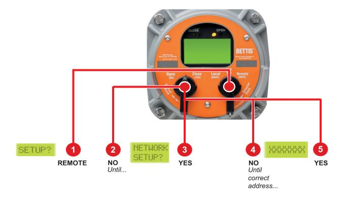
In the **"SETUP"** mode advance to **"NETWORK SETUP?"** using the selector knob in the **REMOTE** position. Answer **YES**. Hold the control knob in the NO position until the correct address appears. Answer **YES**. Unit is now network controlled. If other configuration changes are needed, please see the TEC2 Installation & Operation Manual (E2K-405-0117), which can be found at www.emerson.com/bettis.
