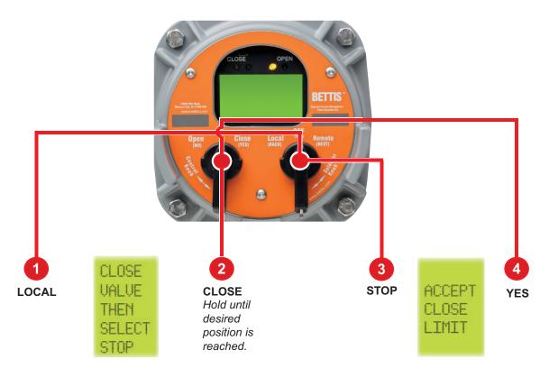
Turn the selector knob to the **"LOCAL"** position. Hold the control knob in the **"CLOSE"** position until desired position is reached. Dis-engage motor drive by setting the declutch lever in **"HAND"** mode. Using handwheel, move the valve in the open direction for one handwheel turn to allow for motor coasting. Re-engage motor drive by setting the declutch lever out of **"HAND"** mode.
