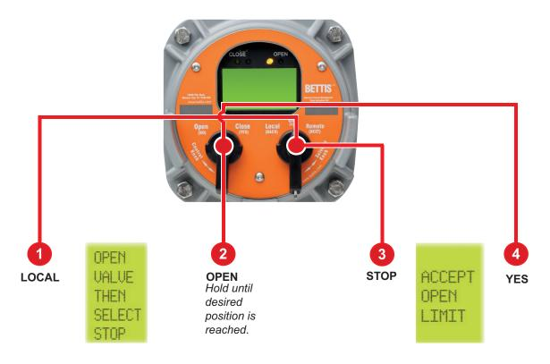
Turn the selector knob to the **"LOCAL"** position. Hold the control knob in the **"OPEN"** position until desired position is reached. Dis-engage motor drive by setting the declutch lever in **"HAND"** mode. Using handwheel, move the valve in the close direction for one handwheel turn to allow for motor coasting.
