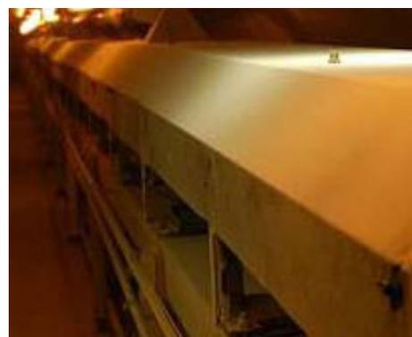
**Image 3.** Each of the nine conveyor belts had four bearing temperature measurements and four rub block temperature measurements that were handled by one Rosemount 848T FOUNDATION Fieldbus High Density Temperature Transmitter.
