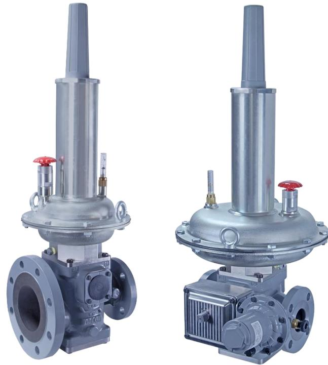
Direct-operated regulators ideal for industrial and commercial applications supplying gas to furnaces, burners and other appliances. A balancing system enables the regulator to control gas pressure accurately for maximum combustion efficiency despite varying inlet pressures.
