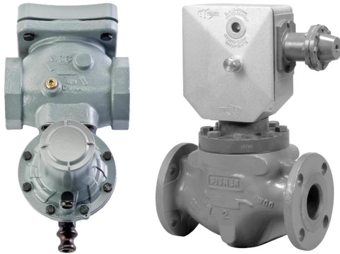
Stand-alone Fisher. slam-shuts offer complete shut-off service without external power supply. Instantaneous shut-off keeps the downstream system from seeing emergency pressure levels.
