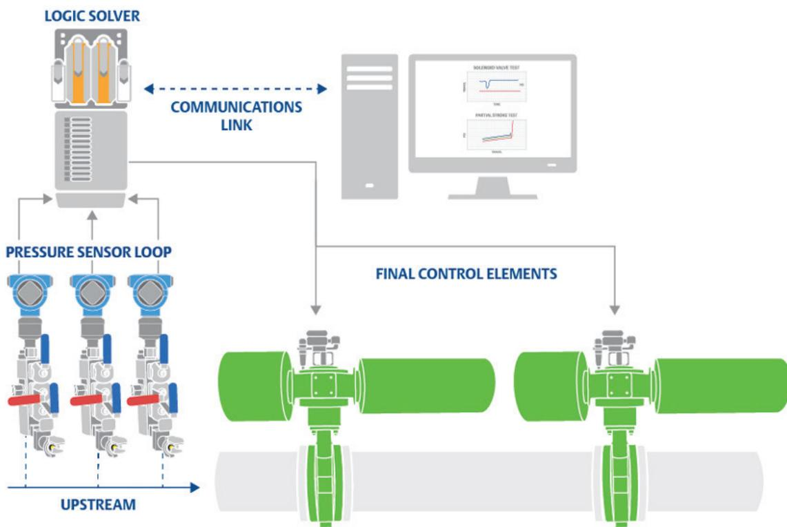
**FIG. 4.** A partial stroke test allows a safety valve to be tested during plant operations. A digital valve controller can safely execute this test, capturing diagnostic data and protecting against inadvertent shutdowns.
