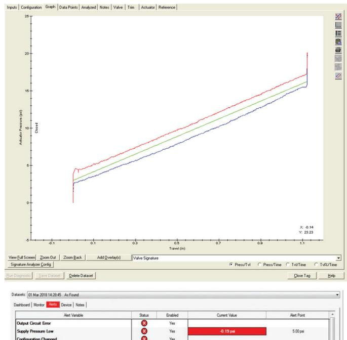
**FIG. 3.** Digital valve controllers incorporate many diagnostics to detect issues with air supply, packing, actuator dynamics and other factors. They also detect actual valve positions.
