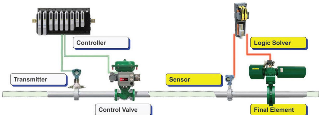
**FIG. 1.** An SIS uses its own sensors, logic solver and final elements—independent of the BPCS—to detect unsafe conditions and protect the plant.
