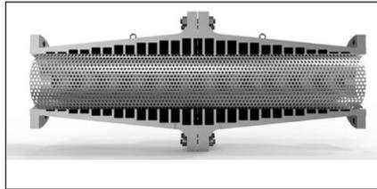
Figure 6. This modal suppressor employs a series of varying sized chambers to generate destructive interference over a range of frequencies, with virtually no pressure drop.
