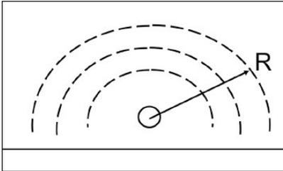
Figure 1B. Control valve noise radiates sound from the pipe itself, as depicted in this piping cross section, so the sound levels drop much more slowly with distance.
