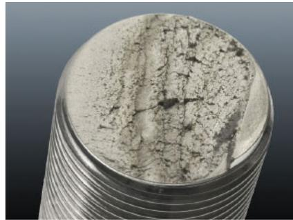
Figure 2. Control valve noise above 110 dBA external to the pipe can fatigue bolts and ultimately crack control valve stems and shafts. For this reason, sound levels should be kept below this threshold.
