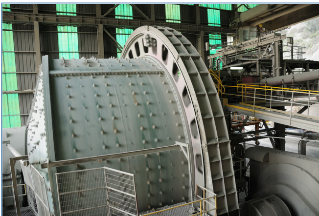
SAG and Ball mills at an ore processing facility – typically the mill drives, the mill gearbox and mill bearings are monitored. Loss of one SAG mill could result in a significant production shortfall.
